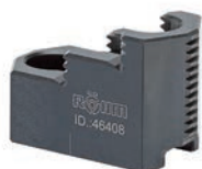
C 21 Reversible top jaws, 3-jaw set, hardened serration 90° - material: 16MnCr5
