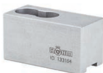
C 21 Soft top jaws, 3-jaw set, can be hardened serration 90° - material: 16MnCr5
